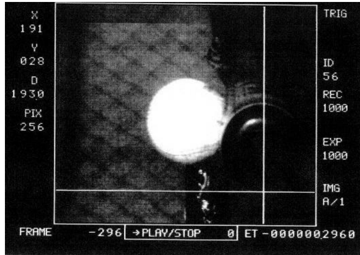
Figure 3. Motion Analysis Capture of a Bat-Ball Impact.
