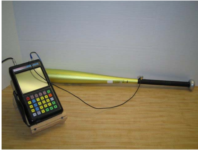
Fig. 4: Measuring the wall-thickness of aluminum bat
