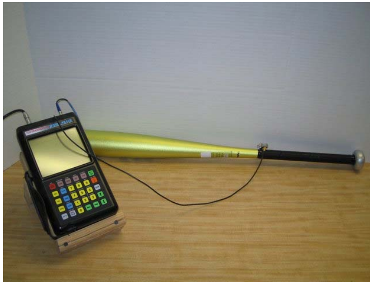
Fig. 15: Wall-thickness measurements with the ultrasonic thickness gage
