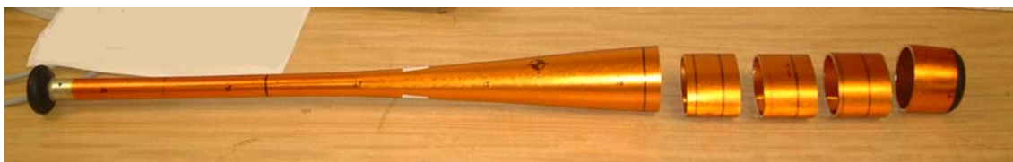
Fig. 13: Three rings taken from the barrel of a bat
