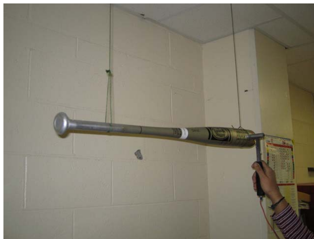
Fig. 19: Impacting a bat with an impact hammer
