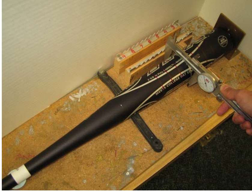
Fig. 8: Measuring the diameter of a bat
