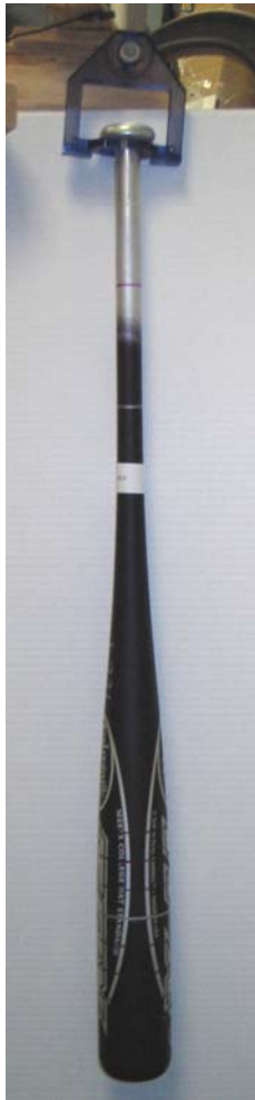
Fig. 9: A bat in pendulum fixture
