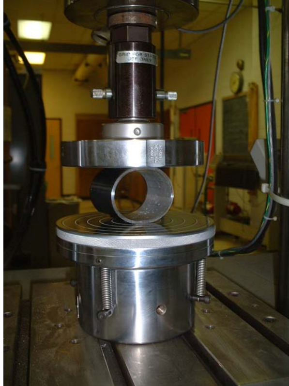
Fig. 14: A ring on an adjustable base for compression test
