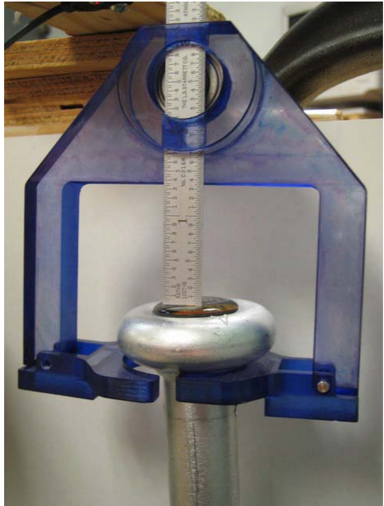
Fig. 10: Measuring the distance from pivot to knob end
