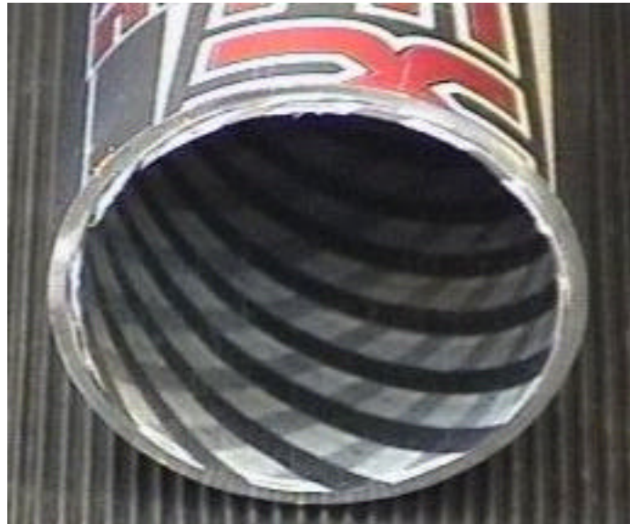
Figure 2.6 – Example of a hollow metal bat with a composite barrel-reinforcement.
