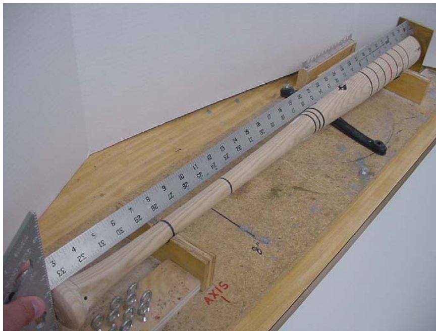
Fig. 7: Use of carpenter's square with profiling station
