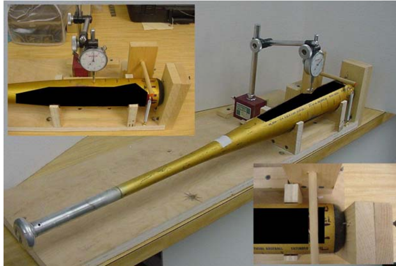
Fig. 12: Surface deformation setup
