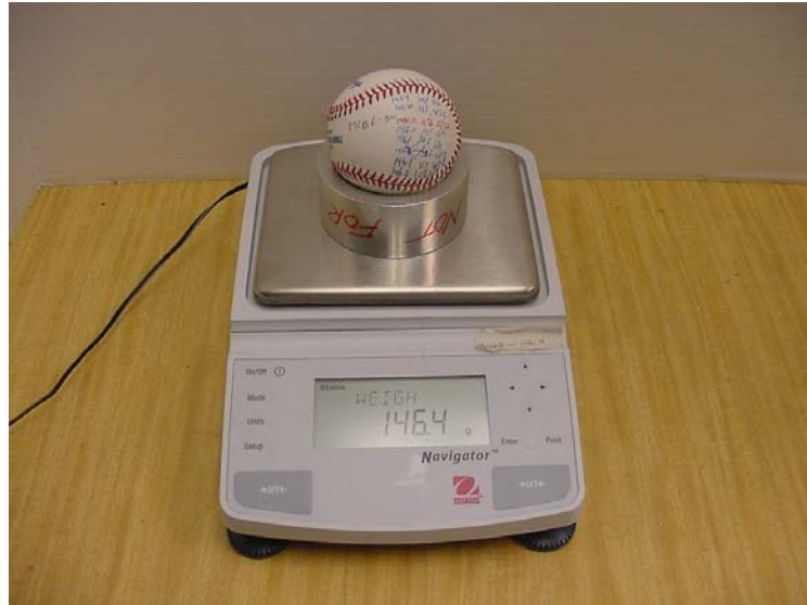
Fig. 8: Ohaus scale measuring weight of a baseball
