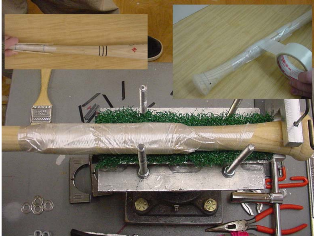
Fig. 16: Wrapping of handle of wood bat for reinforcement
