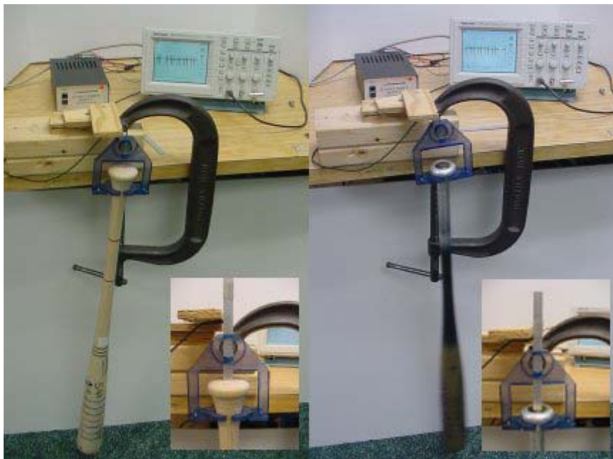
Fig. 10: MOI fixture showing both wood and aluminum bats
