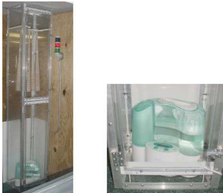
Fig. 17: Humidity chamber (left) and humidifier (right)
