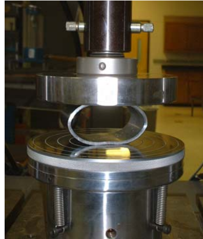
Fig. 3 Barrel compression test on a ring by an Instron machine.
